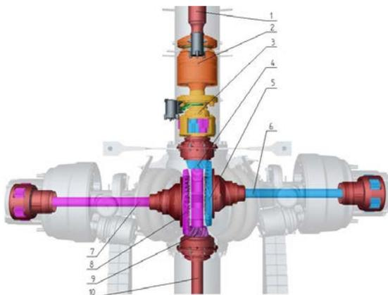
Figure 1. Distribution of the drive torque to the axles
