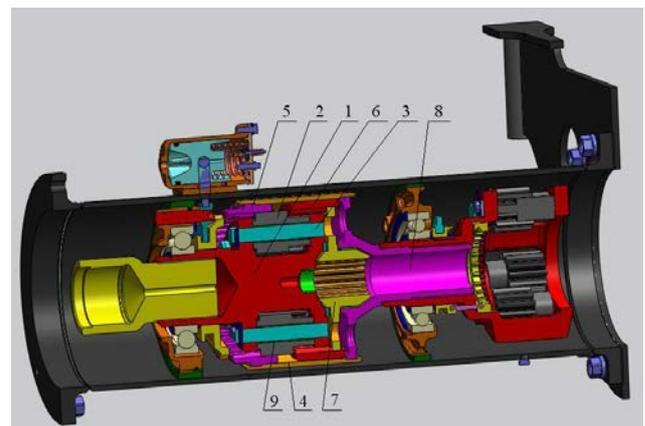
Figure 2. The basic center differential in the rear-axle tube
