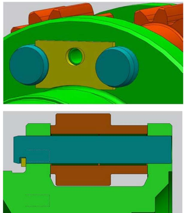
Figure 11. Designed geometrical modification of lock plate
