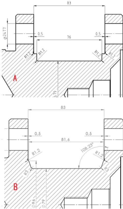
Figure 7. Designed geometrical adjustment of housing: A - original shape, B - designed shape
