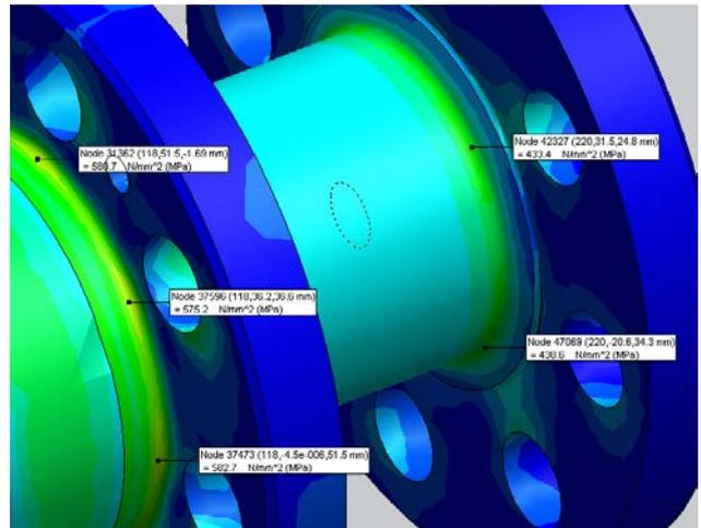
Figure 9. Stress in selected nodes after geometry optimization
