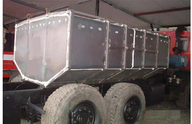
Figure 17. The made water tank on the truck
