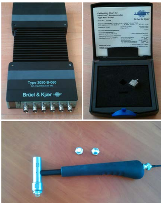
Figure 3. Modul Pulse, monoaxial accelerometer and modal hammer [7]
