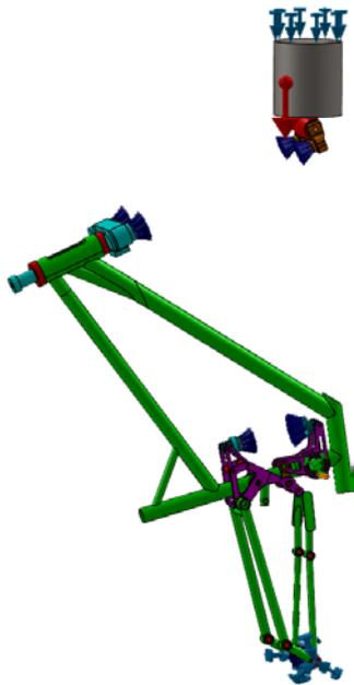
Figure 5. Geometrical model and boundary conditions for impact test 1
