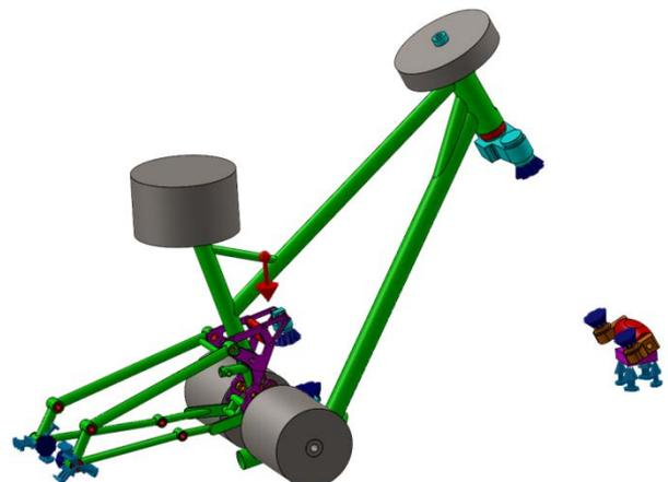
Figure 9. Geometrical model and boundary conditions for impact test 2
