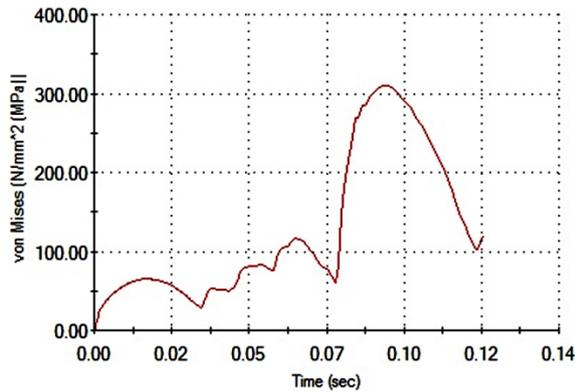
Figure 11. The time dependence of maximum reduced stress
