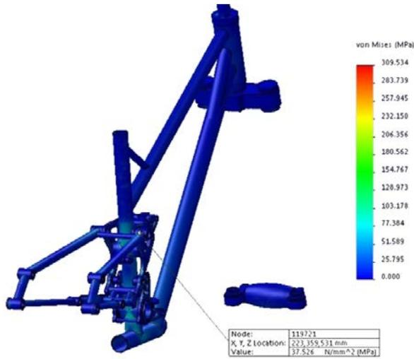
Figure 10. The field of maximum reduced stress at the time 0.09 s
