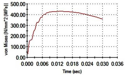
Figure 7. The time dependence of maximum reduced stress
