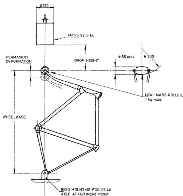
Figure 3. Setup of impact test: Drop mass [3]
