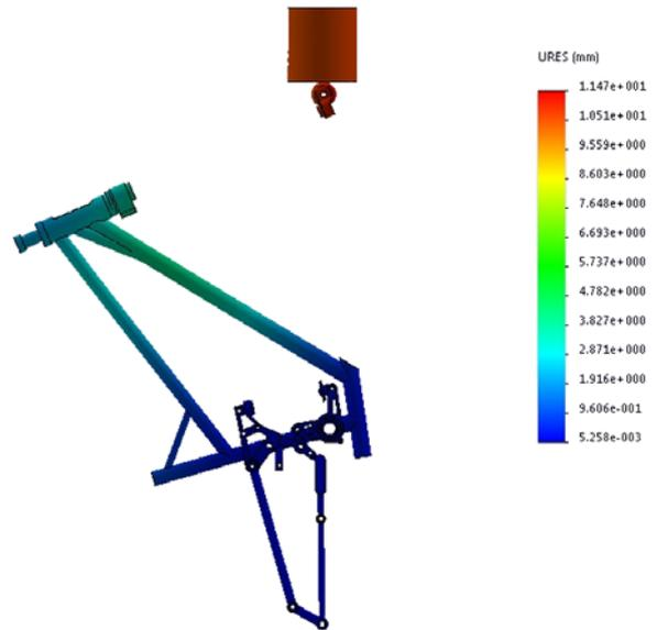
Figure 8. Displacement field at the time 0.012 s
