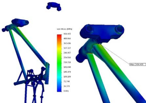
Figure 6. The field of maximum reduced stress at the time 0.012 s
