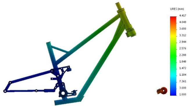
Figure 12. Displacement field at the time 0.012 s
