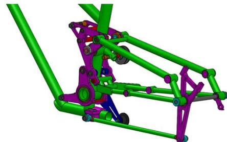
Figure 2. Suspension of rear triangle
