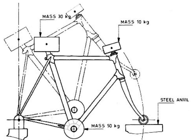
Figure 4. Setup of impact test: Frame drop [3]
