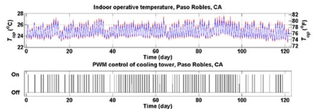
Figure 6. Operative temperatures and PWM when cooling tower deadband interval is 1 °C
