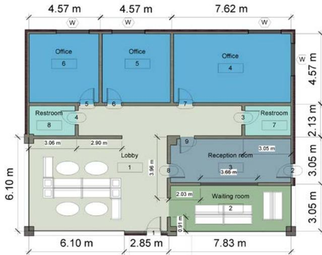
Figure 2. Floor plan of the small commercial building
