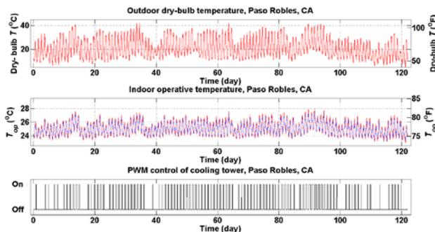
**Figure 8. Temperatures and PWM control in Paso Robles, CA**
