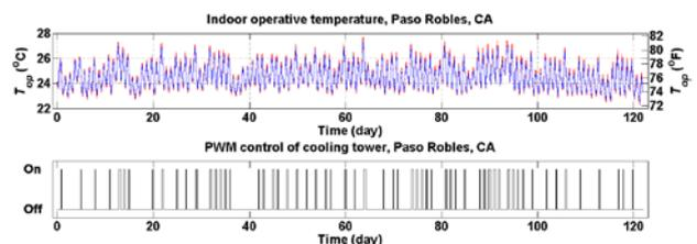
Figure 7. Operative temperatures and PWM when cooling tower deadband interval is 2 °C
