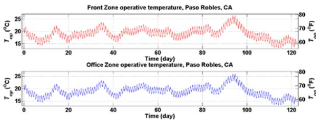
Figure 4. Operative temperatures in the summer of 2007 while cooling tower worked fully
