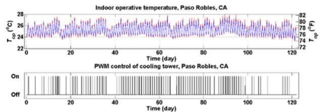
Figure 5. Operative temperatures and PWM when cooling tower deadband interval is 0 °C
