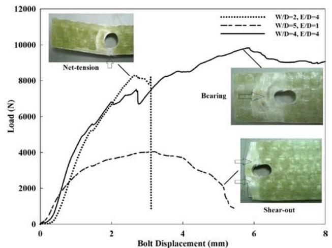
Figure 5. Failure modes based on the different responses when the bolted joints were subjected to bearing test
