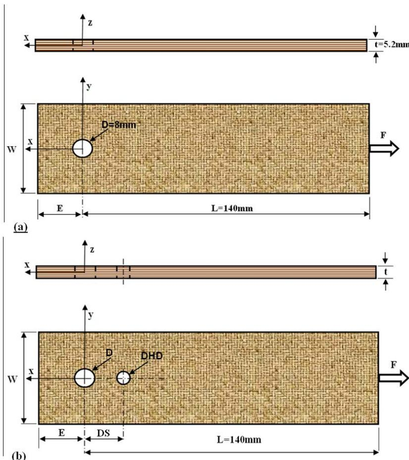
**Figure 1.** The geometry of the laminate test coupons; (a) without the DHS, and (b) with the DHS
