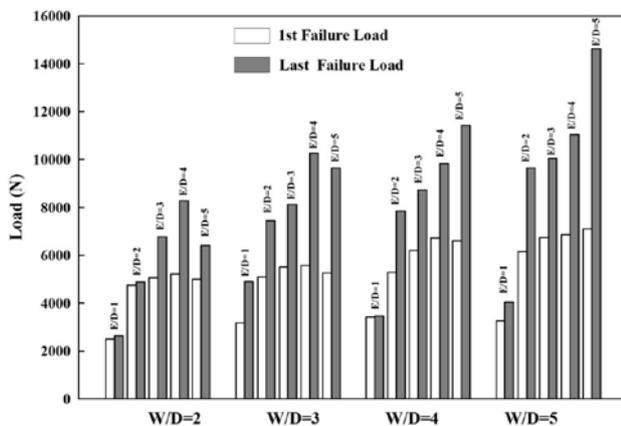
Figure 4. The failure loads experienced by the laminates following the bearing tests
