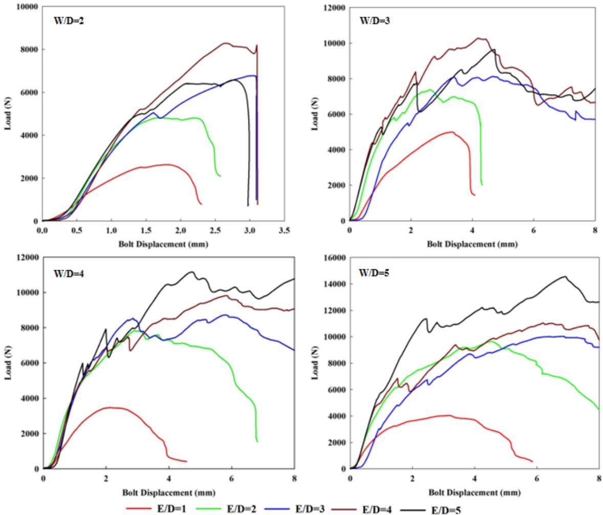
**Figure 3.** Load-displacement curves for the bolted joints with different configurations
