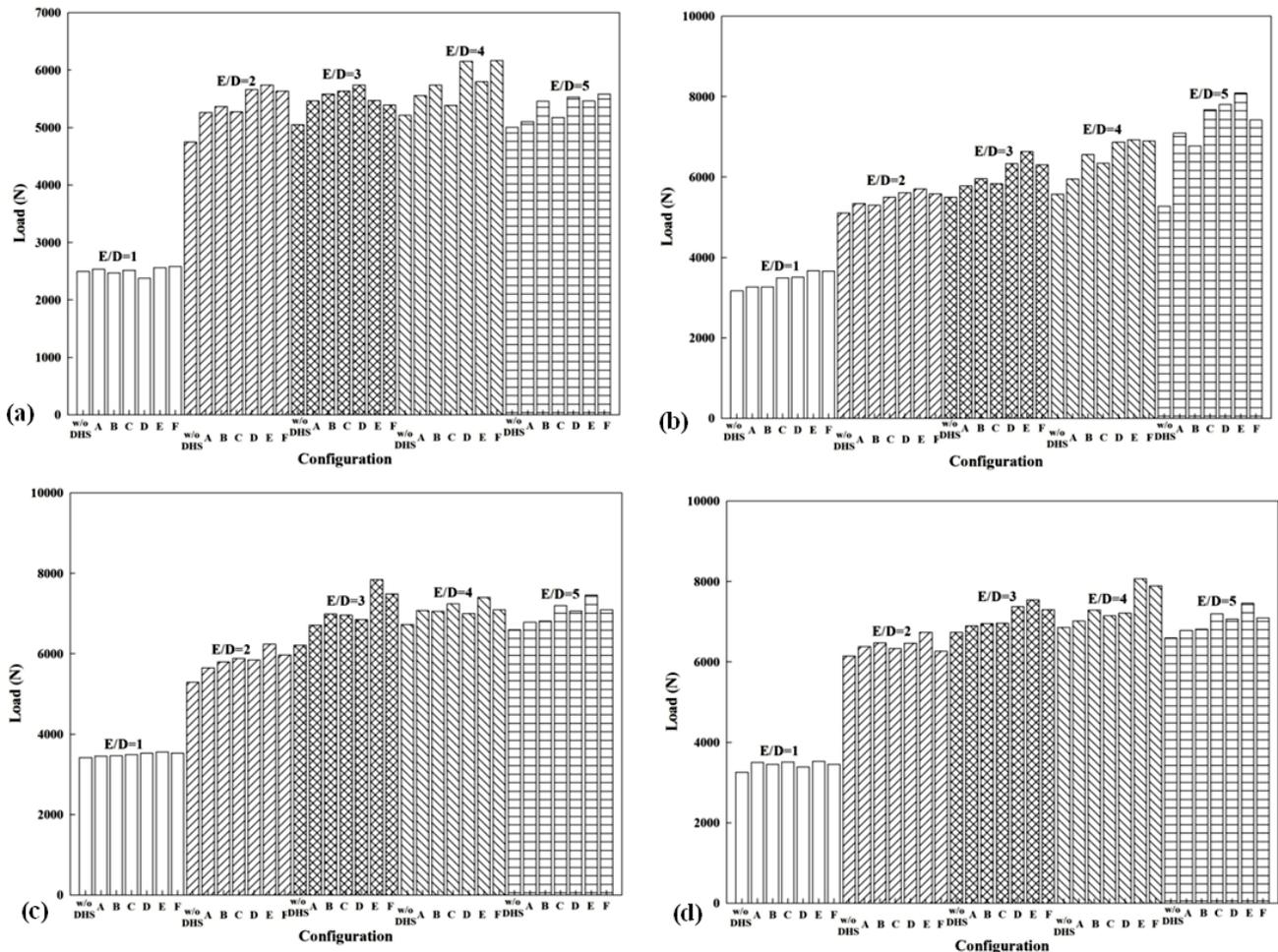
**Figure 6.** Failure loads of the composite bolted joints with (a) W/D=2; (b) W/D=3; (c) W/D=4; and (d) W/D=5
