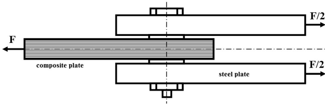
**Figure 2.** Schematic of the composite bolted joint for the bearing test
