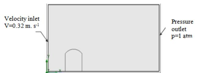
Figure 2. Boundary conditions in the test section
