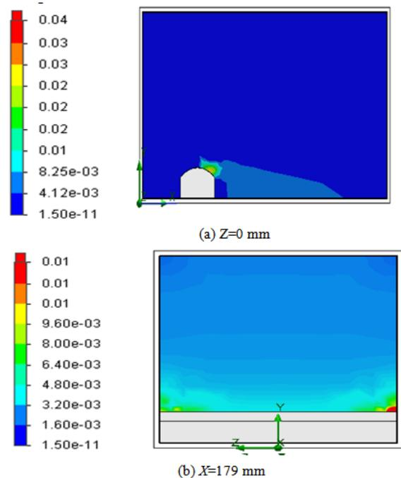
Figure 8. Distribution of the turbulent dissipation rate
