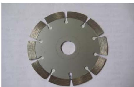
Figure 1. Sample of circular Tile-Cutter
