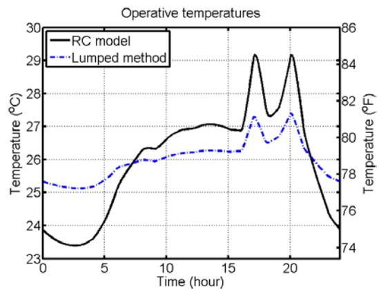
**Figure 9.** Operative temperatures by using the RC model and the lumped method
