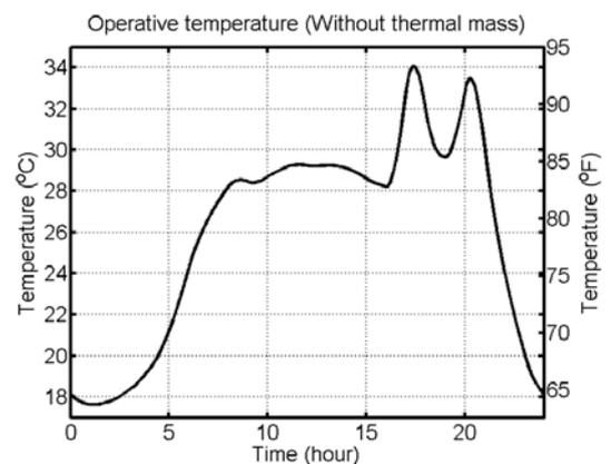
**Figure 10.** Operative temperature in the extreme case without thermal mass
