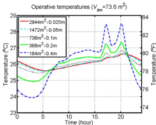
Figure 12. Operative temperatures of changing the heat transfer rate between the iTM and the indoor air
