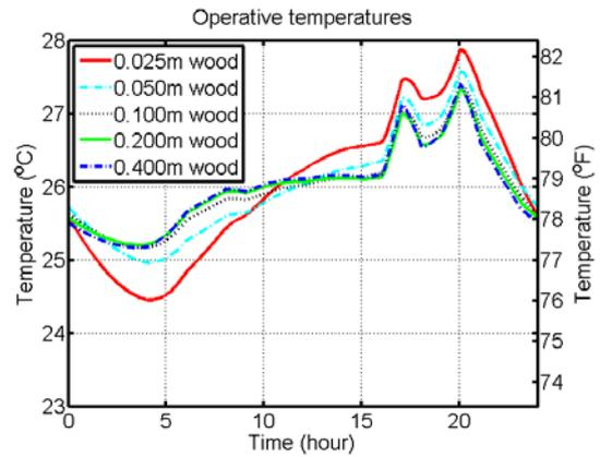
Figure 7. Operative temperatures of the wood house with different wood thicknesses
