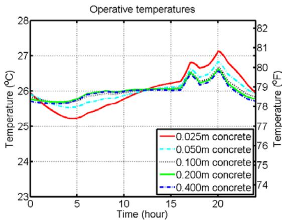
**Figure 8.** Operative temperatures of the concrete house with different concrete thicknesses
