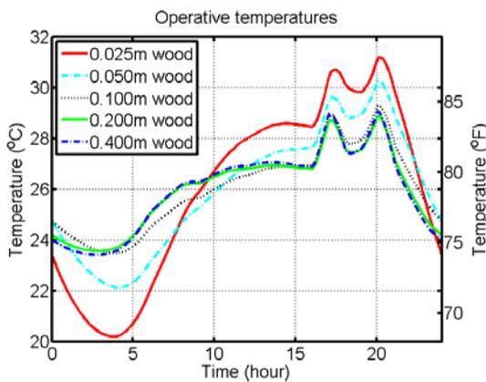
Figure 11. Operative temperatures when changing the iTM size (thickness)
