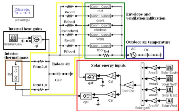
Figure 5. RC model of the house in Matlab/Simulink
