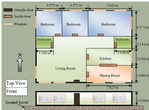
Figure 1. Schematic of the prototypical residential house
