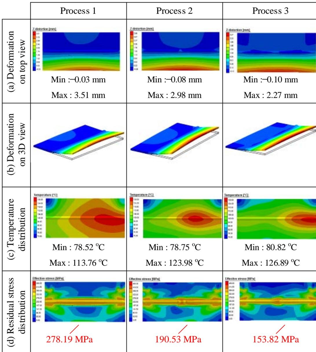
Figure 6. Simulation results at the end of the welding cycle
