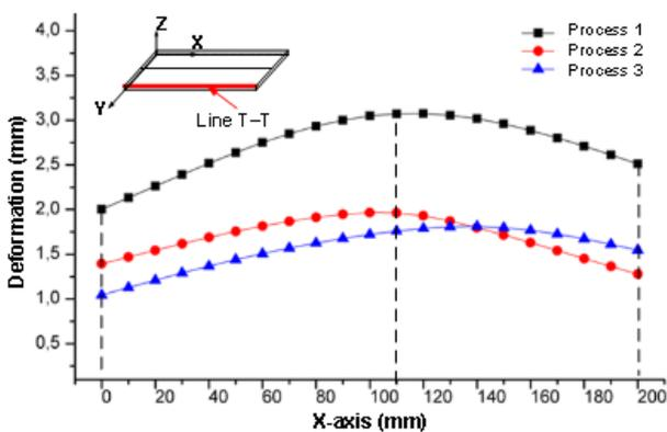
Figure 7. Simulation result of plate deformation on line T-T
