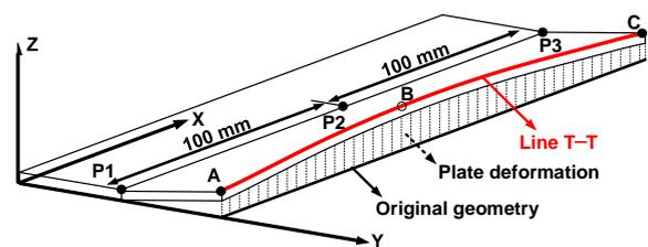
Figure 4. Location for observing the welding deformation
