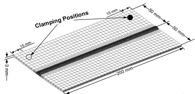
Figure 3. Mesh model for simulation
