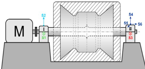
Figure 3 .Locations and measurement directions of accelerometers
