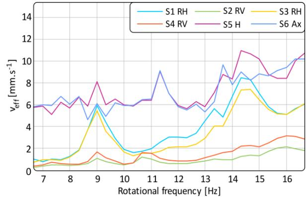
Figure 4. Effective vibration velocity as function of rotation frequency
