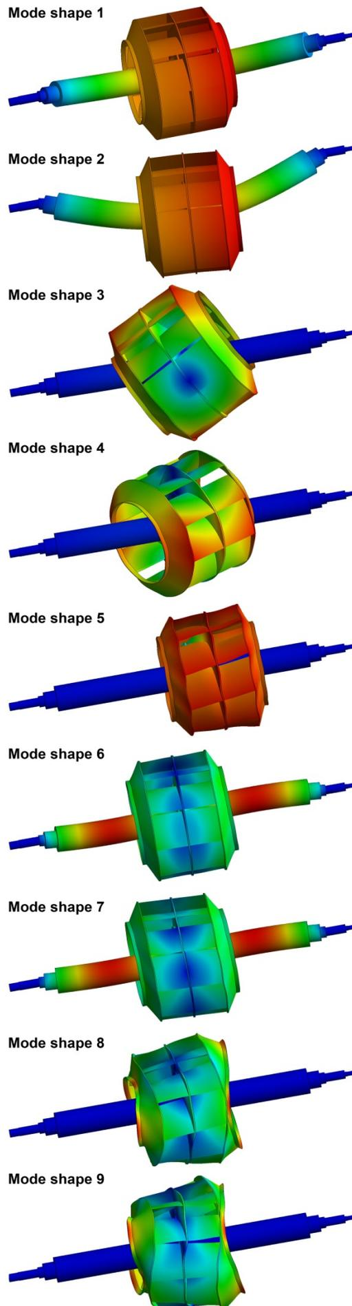
Figure 9. Mode shapes of the analyzed model at 1000 rpm
