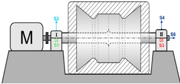
Figure 6. Locations and directions of measured responses
