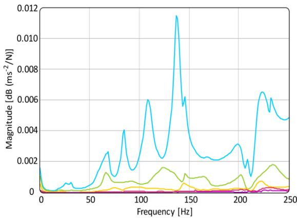
Figure 7. Complex Mode Indicator Function of the analyzed structure
