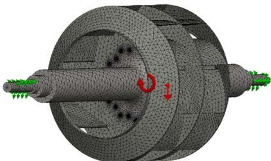
Figure 8. Finite element mesh of the numerical model
