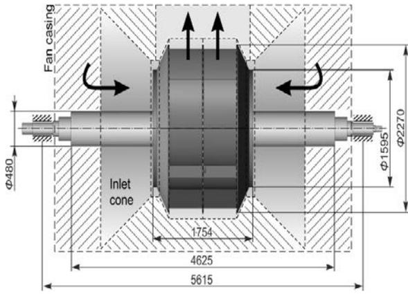
Figure 2. Basic dimensions of the impeller and shaft
