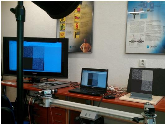
Figure 1. Configuration of the 3-D correlation system with investigated patterns bonded on a flat specimen
