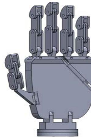
Figure 7. 3D model of humanoid robot hand
