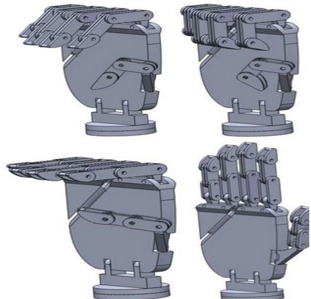
Figure 8. Motion possibilities of designed humanoid robot hand
