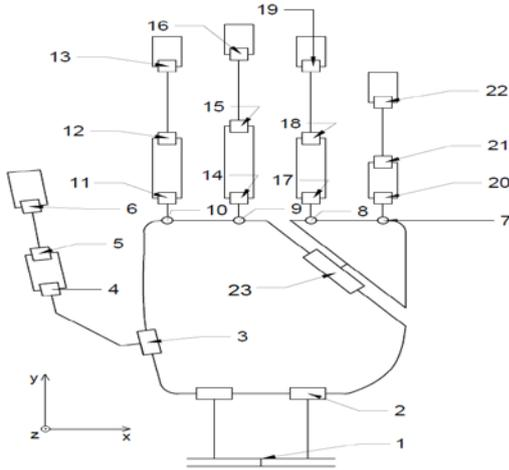
Figure 3. Kinematic configuration of humanoid hand
