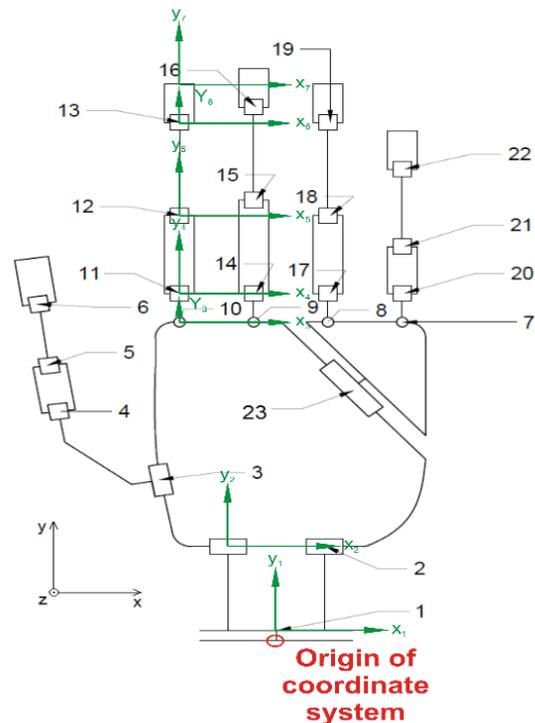
Figure 4. Coordinate systems of humanoid robot hand
