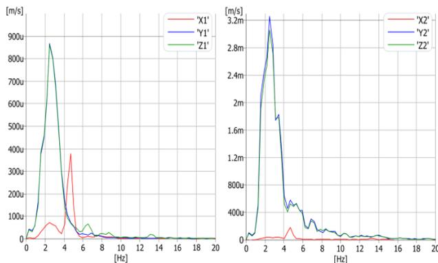
Figure 12. Frequency spectrum of maximum vibration velocities of non-moving railcar measured by sensors S1 and S2
