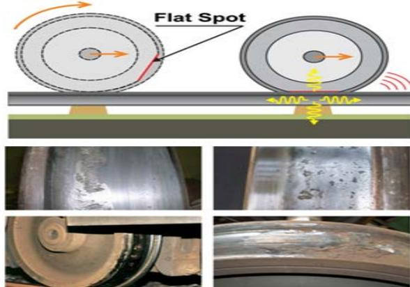
**Figure 4.** Damage of railcar wheel
