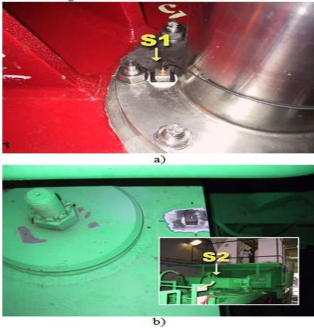
Figure 6. a) Location of sensor S1 on lid of container, b) location of sensor S2 on the frame of undercarriage over bearing shell of wagon
