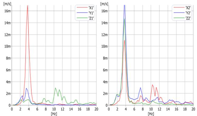
Figure 7. Section No. 1 - acceleration through railway switches
