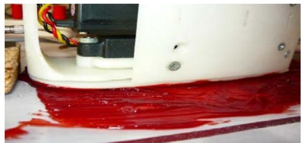
Figure 11. Layer of lubricant before snake robot segment
