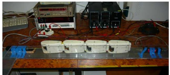
Figure 6. Measuring of friction on snake robot LocoSnake
