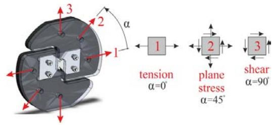
Figure 4. State of stress under load in different directions
