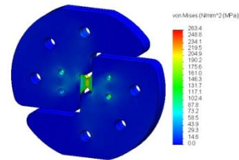
Figure 10. The fields of reduced stress  $\sigma_{red}^{HMH}$  on the assembly
