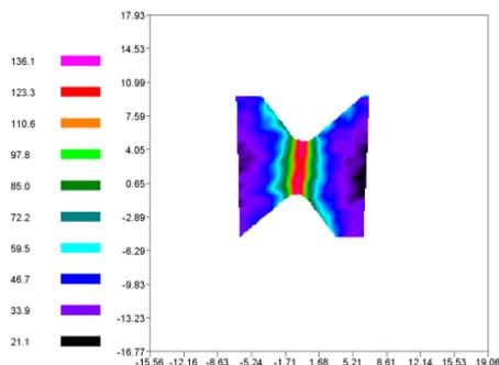
Figure 16. Reduced stress fields  $\sigma_{red}^{HMH}$
