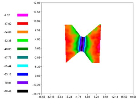
Figure 17. Tangential stress fields  $\tau_{xy}$
