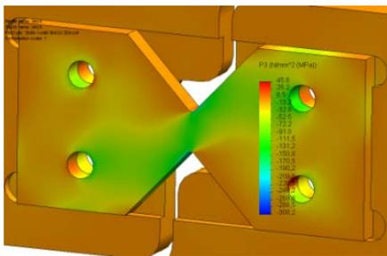
Figure 14. The principle stress fields  $\sigma_3$
