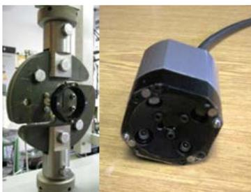
Figure 9. Fixture with the experimental sample and the optical sensor Q 100
