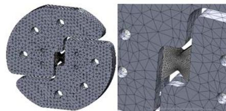
Figure 6. Finite element mesh and detail the mesh in the middle area of the experimental sample with V notch
