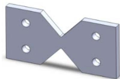
Figure 1. The experimental sample with a symmetric V notch
