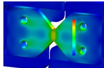
Figure 11. Reduced stress fields  $\sigma_{red}^{HMH}$
