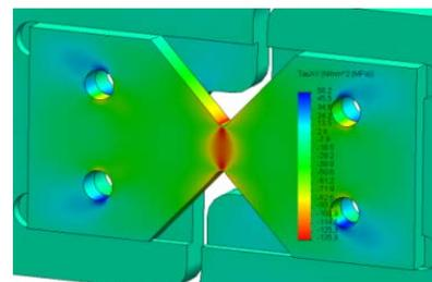
Figure 12. Tangential stress fields  $\tau_{xy}$
