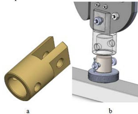
Figure 5. Coupling tension machine with fixture
