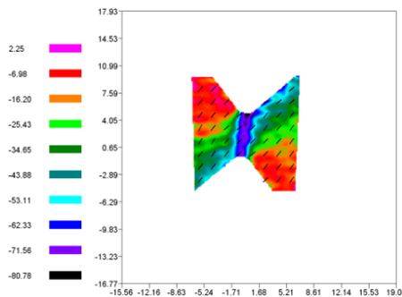
Figure 19. The principle stress fields  $\sigma_3$  with their direction orientation
