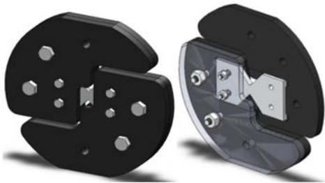
Figure 3. Fixture with bolt connections in Solid Works
