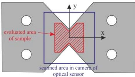
Figure 15. Scanned area of experimental sample (ESPI method)
