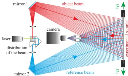
Figure 7. Measuring In Plane - ESPI
