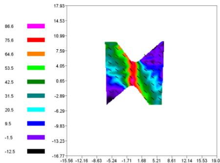
Figure 18. The principle stress fields  $\sigma_1$  with their direction orientation
