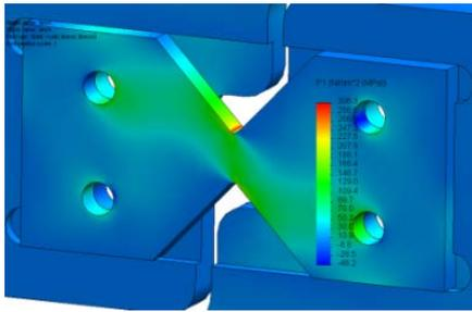
Figure 13. The principle stress fields  $\sigma_1$
