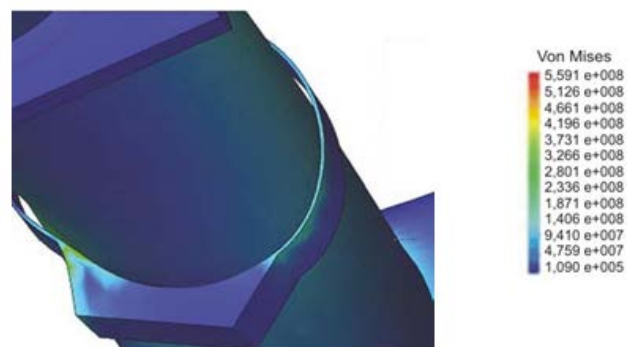
Figure 15. Detail of stresses in foot
