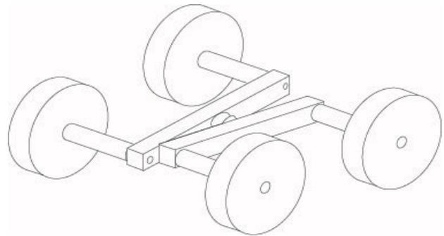
Figure 11. Simple longitudinal rocker [2]
