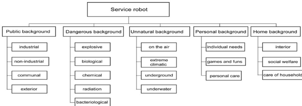
Figure 2. Space of application service robots [1]
