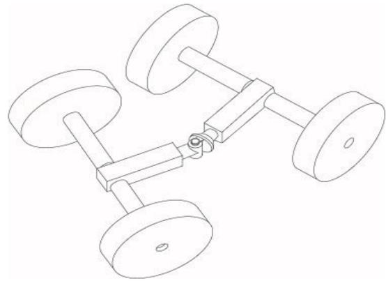
Figure 10. Two-section connected through vertical joint [2]
