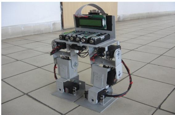
Figure 1. Two legged robot Wirgil
