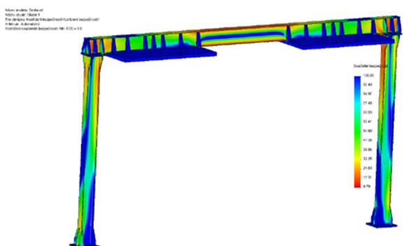
Figure 12. Layout of the safety factor (option No. 1)
