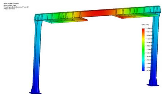
Figure 10. The resulting displacements field (option No. 1)
