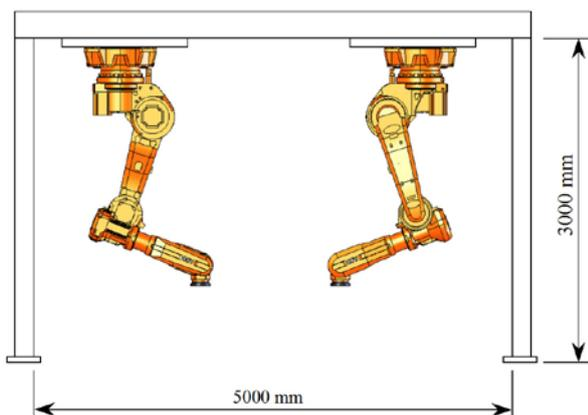
Figure 4. Base required dimensions of the portal structure
