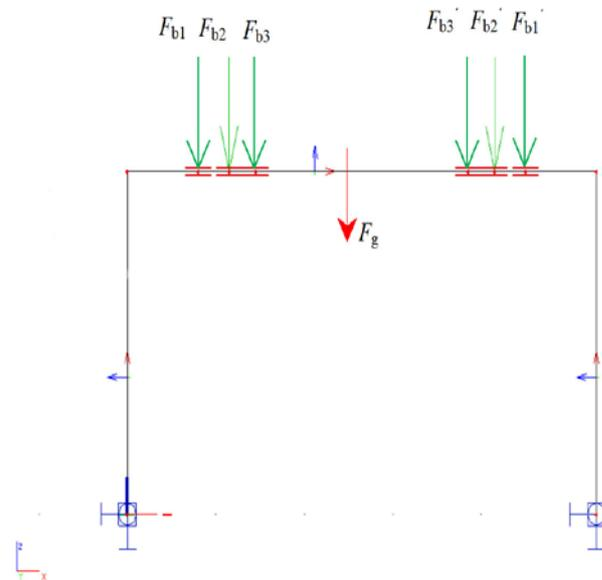
Figure 5. Adverse grouping of forces acting to the robot in SCIA engineering software (option No. 1)
