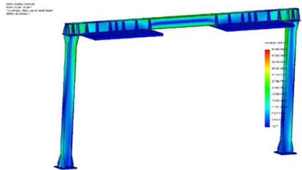
Figure 9. Von Mises stress field (option No. 1)
