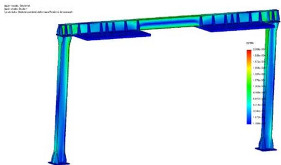
Figure 11. Field of strains (option No. 1)
