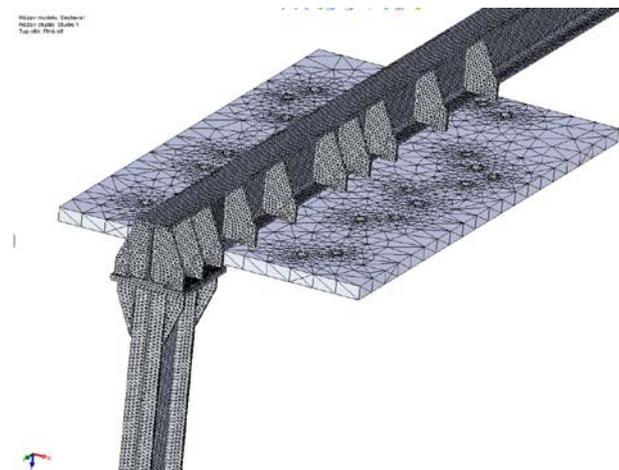
Figure 8. Volume network created on the geometric model (option No. 1)
