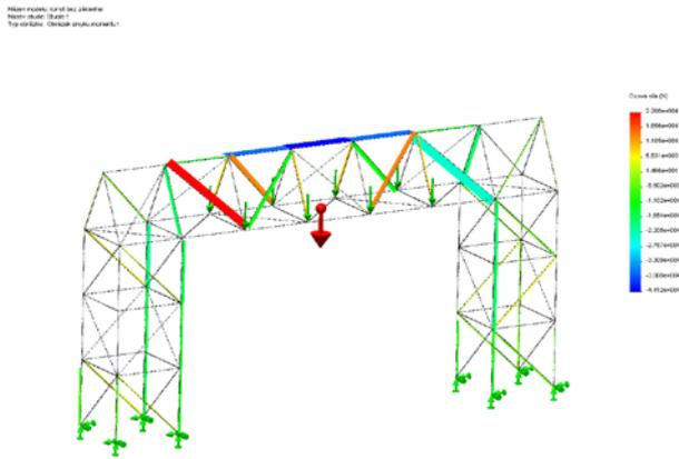
Figure 18. Axial forces in the rods (option No. 2)
