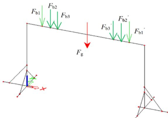
Figure 20. Adverse grouping of forces acting to the robot in SCIA engineering software (option No. 3)
