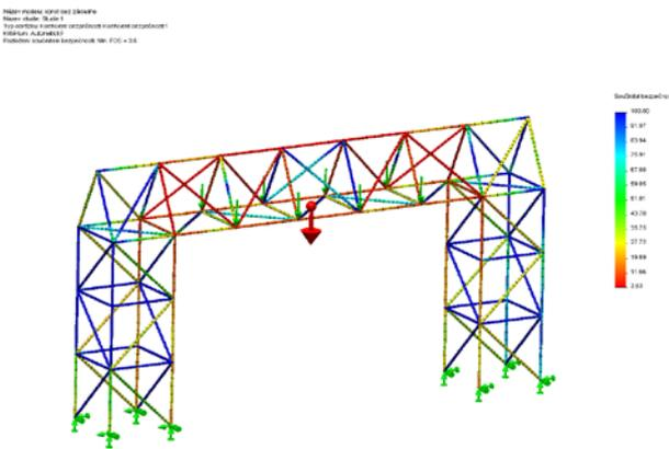
Figure 19. Layout of the safety factor (option No. 2)
