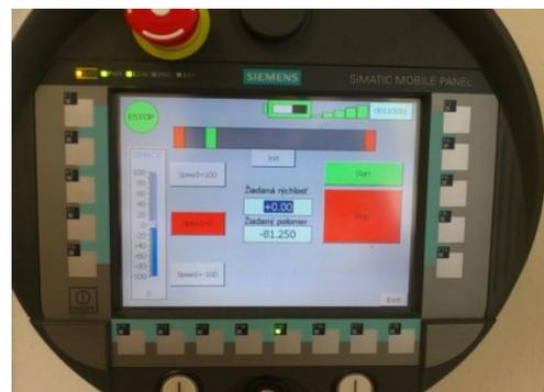
Figure 12. SIMATIC mobile panel 277F IWLAN
