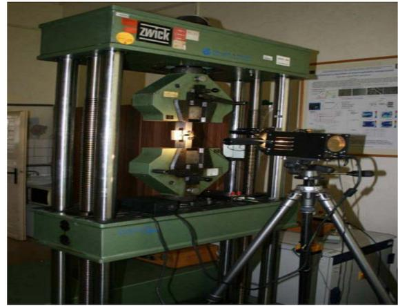
**Figure 3.** Tearing machine Zwick 1387 with reflection polariscope LF/Z-2
