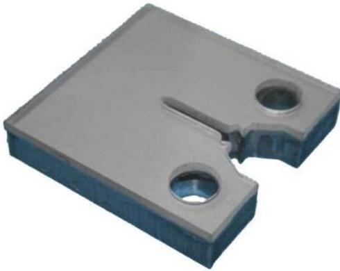
**Figure 2.** Analysed sample with photoelastic coating PS-1A
