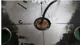
Figure 4. Milled ring core
