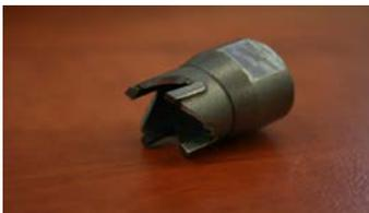
Figure 5. Hollow mill
