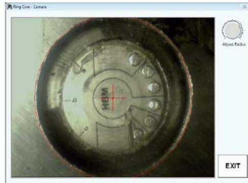
Figure 11. Centering the mill
