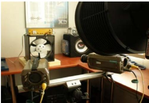
Figure 4. Configuration of the 3-D image correlation system with investigated cooling fan
