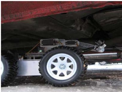
Figure 2. Mobile robot with sectional undercarriage
