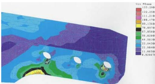
Figure 5. Detail of distribution of stresses in [MPa]
