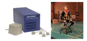
Figure 2. The magnetic motion capture Nest of Birds [1]
