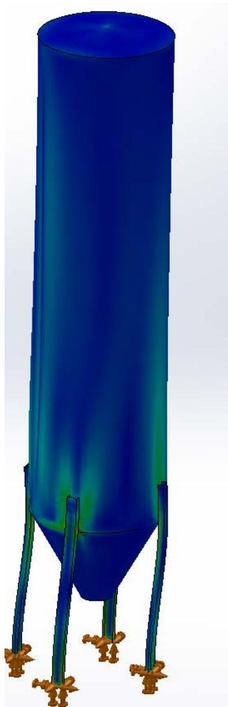
Figure 9. The process of the Von Misse stress
