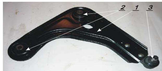
**Figure 2.** Steel control arm: 1-drawpiece, 2- rubber-metal bushing, 3-spherical pin
