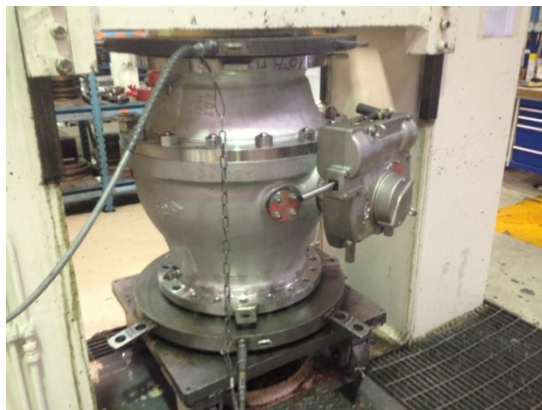
Figure 2. Full bore ball valve, soft seat 20" CL150, 22Cr duplex body (Face-to-face: 914 mm, Weight: 1569 KG)
