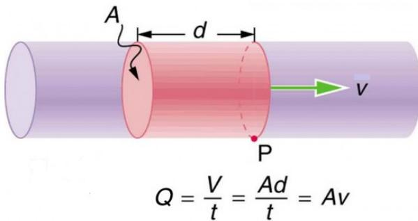
Figure 5. Velocity of the fluid in the pipe
