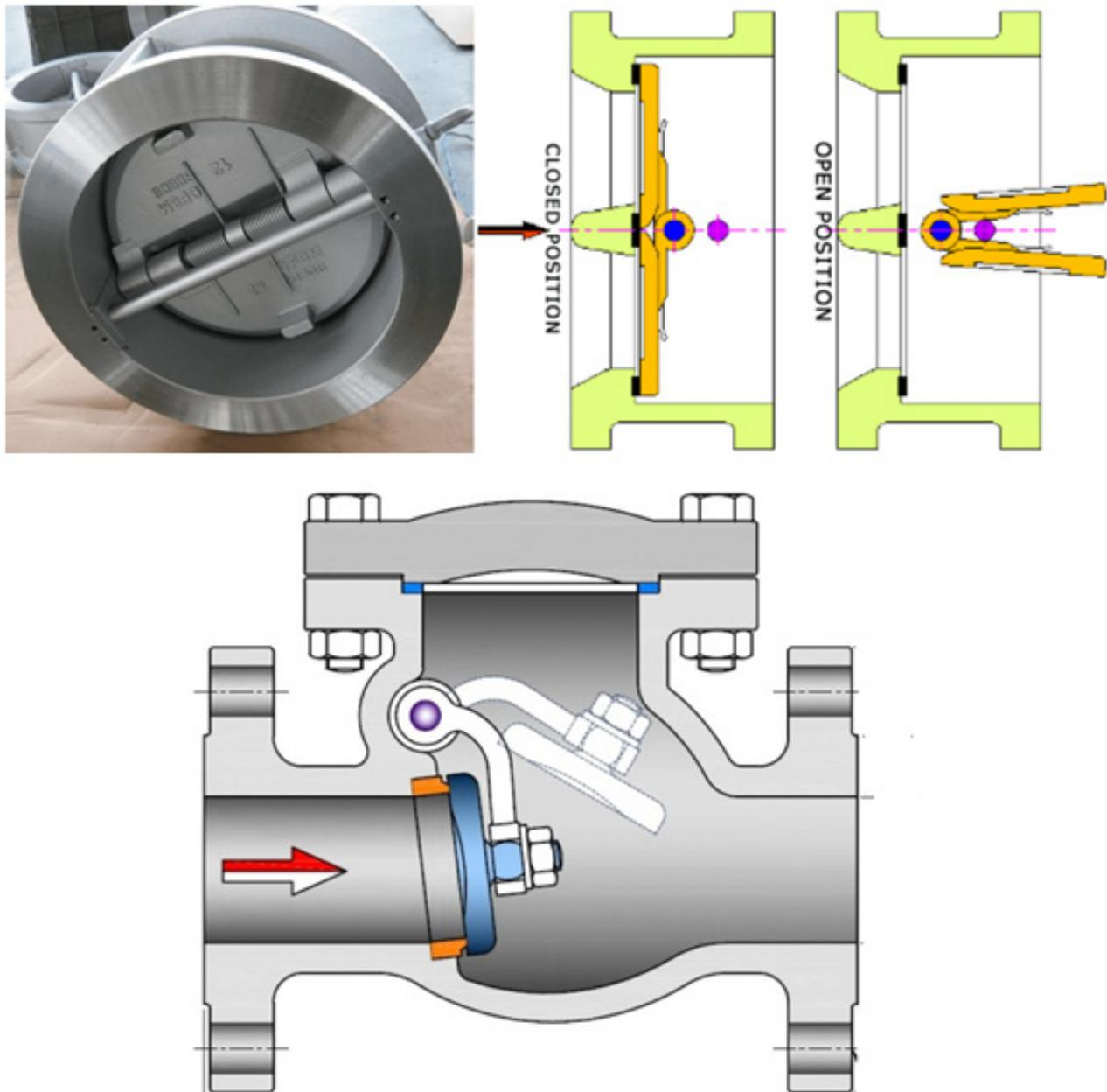
Figure 2. Comparison between swing and dual plate check valve
