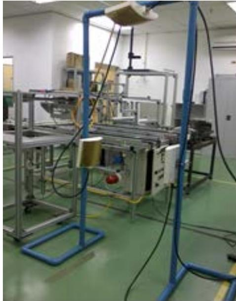
Figure 3. Experimental setup showing the RFID gate with three antennas
