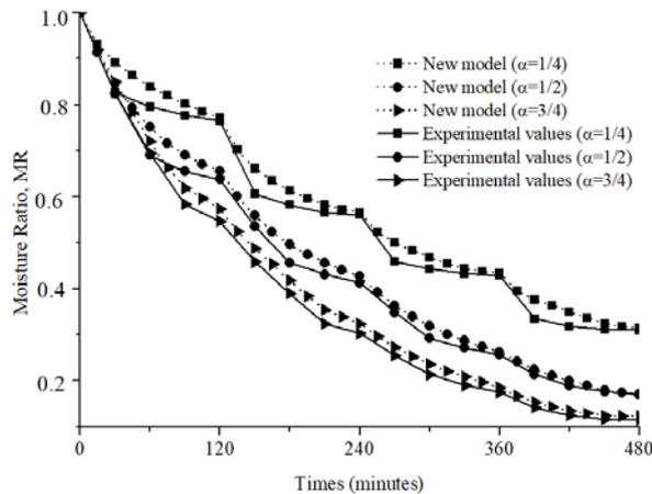
**Figure 3.** Comparison of the experimental profiles and the simulated model of the moisture ratio of mango during intermittent drying at 50°C
