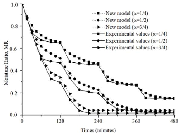
**Figure 4.** Comparison of the experimental profiles and the simulated model of the moisture ratio of mango during intermittent drying at 60°C
