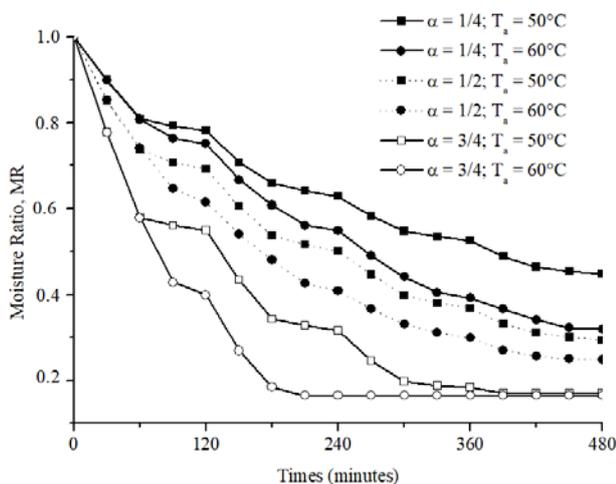
**Figure 2.** Influence of intermittency on the moisture ratio of mango samples at 50 and 60°C
