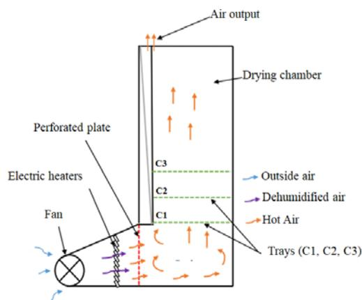
Figure 1. The electrical laboratory modular dryer
