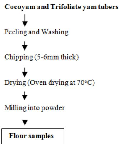
**Figure 2.** Flow chart for the production of cocoyam flour and trifoliate yam flour. Source: [17]
