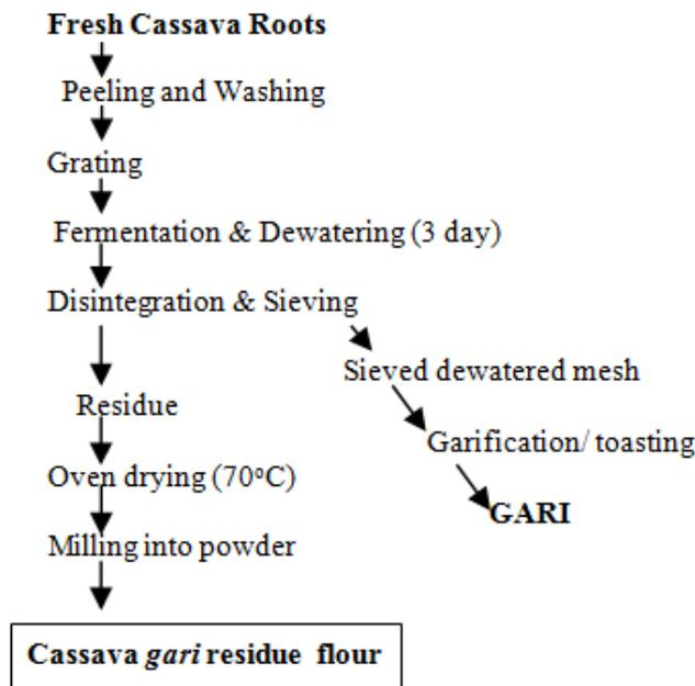
**Figure 1.** Flow chart for production of cassava residue flour obtained from *gari* processing operation. Source: [16]
