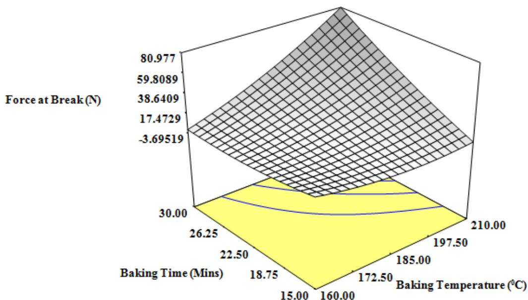
Figure 2. Effect of baking time and temperature on force at break of cookies
