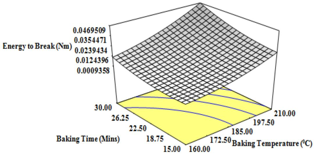
Figure 3. Effect of baking time and temperature on energy to break of cookies
