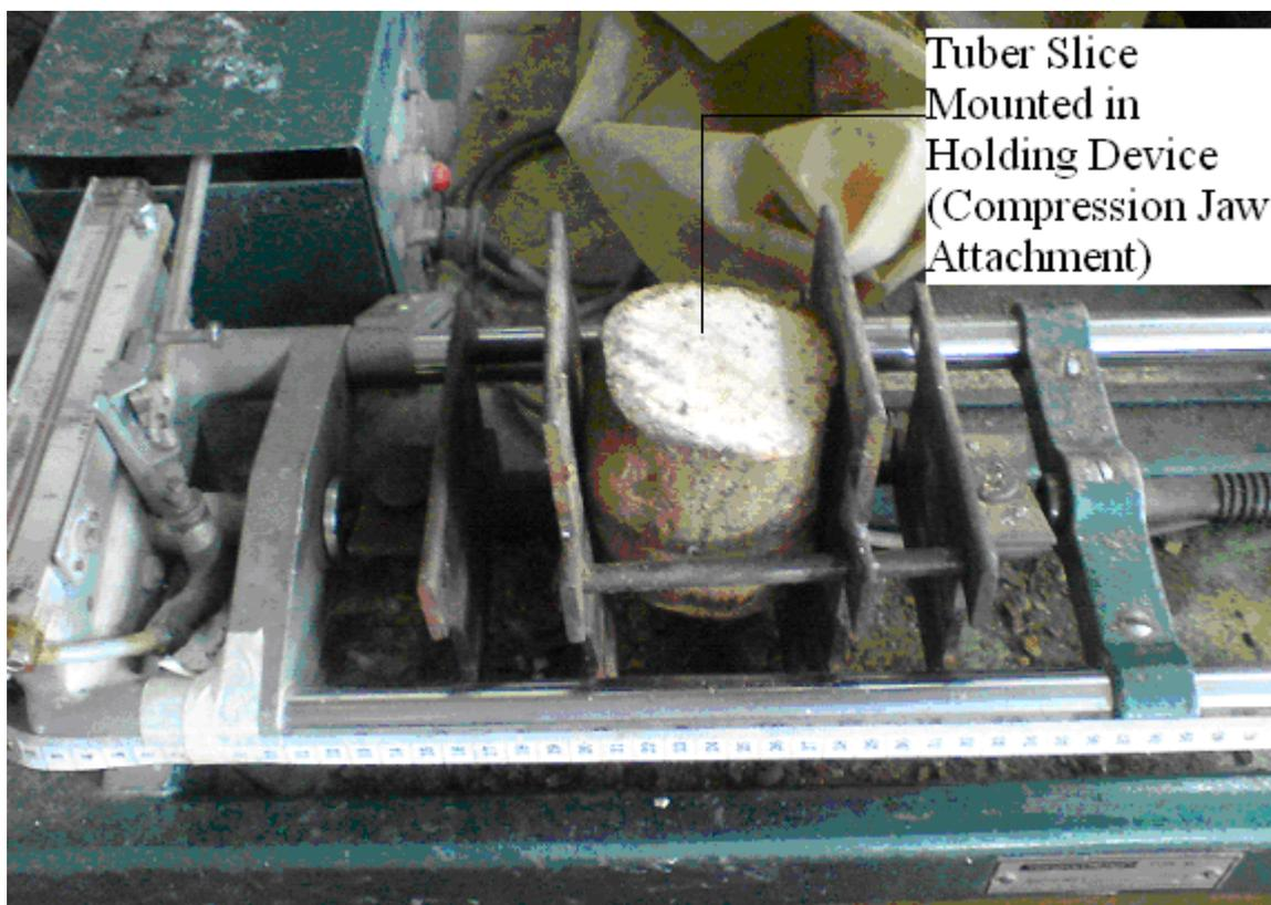
Figure 1. Length of tuber slice inserted in the holding device of the adapted Tensometer
