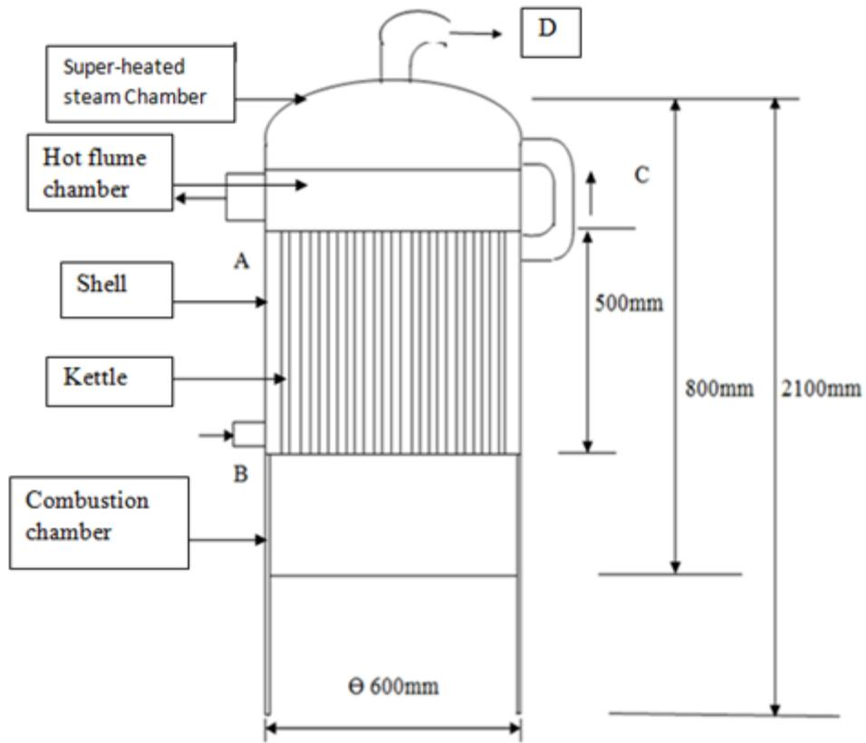
Figure 1. Schematic diagram of biomass fire-in-tube boiler
