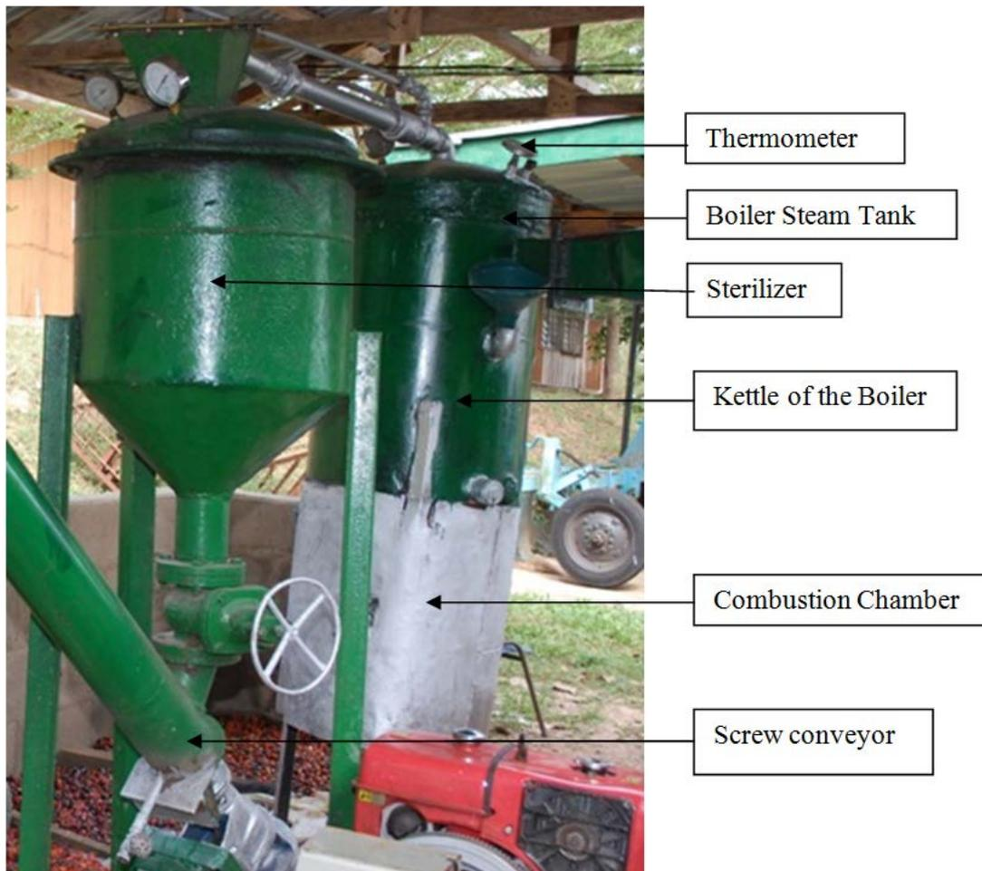
Figure 2. Vertical Sterilizer synchronized with Biomass boiler
