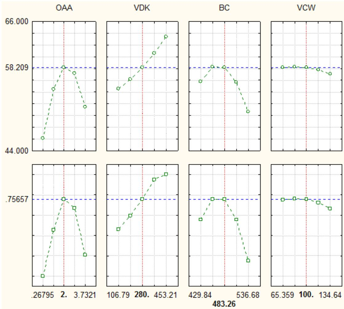
**Key:** OAA – Orifice Area of Aspirator, VDK – Vertical Distance of Fire-grate to the bottom of kettle, BC – Biomass Composite, VCW – Volume of cold water inside kettle.
