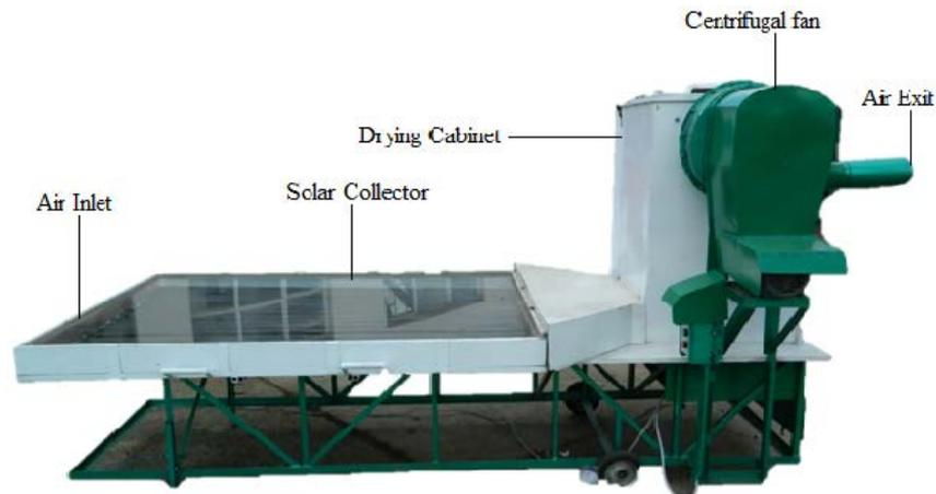
Figure 1. Side View of Experimental solar dryer
