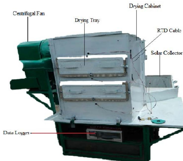
Figure 2. Rear View of Experimental Solar dryer
