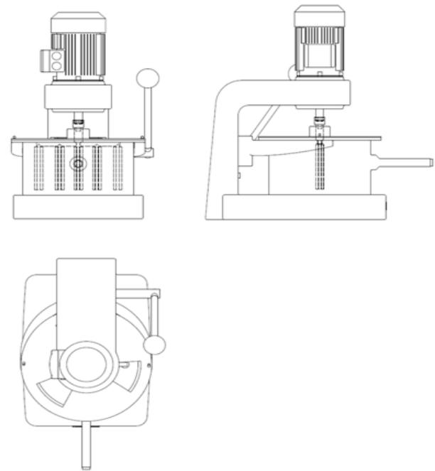
**Figure 3a.** Orthographic view of the cowpea dehuller with vertical beaters
