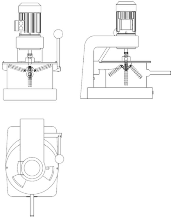
**Figure 2a.** Orthographic view of the cowpea dehuller with inclined beaters
