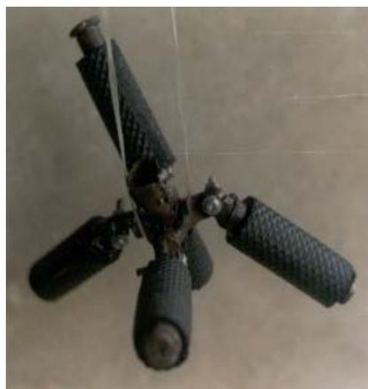
**Figure 5a.** The rubber-lined inclined beaters
