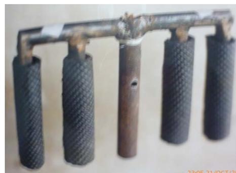
**Figure 5b.** The rubber-lined vertical beaters
