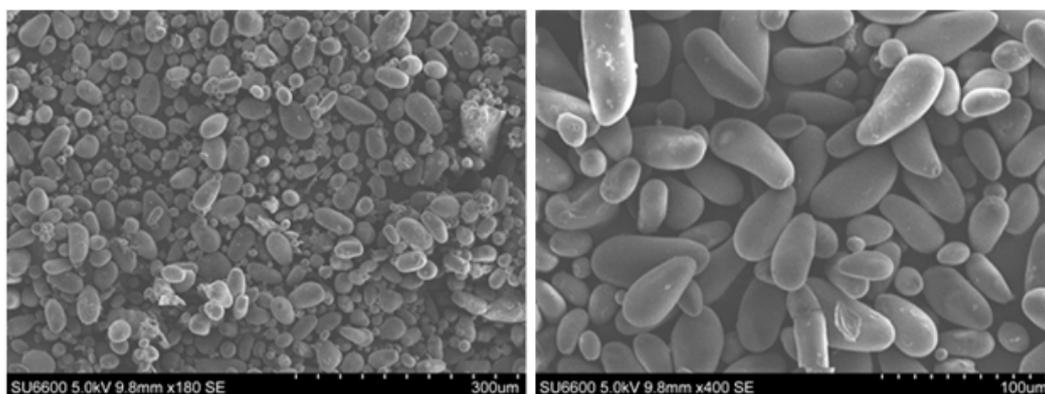
**Figure 6.** Scanning Electron Micrograph (SEM) of Native Kithul (*Caryota urens*) flour under two magnifications (300µm and 100 µm)
