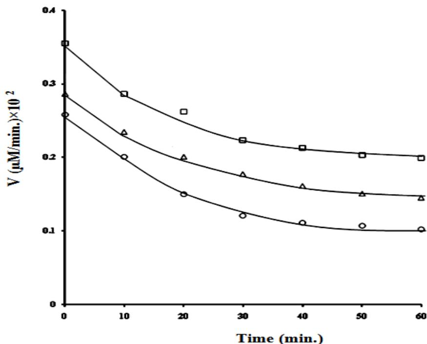
Figure 6. Thermal denaturation of the enzyme at different temperatures. (45 °C (□), 50 °C (Δ) and 55 °C (o))
