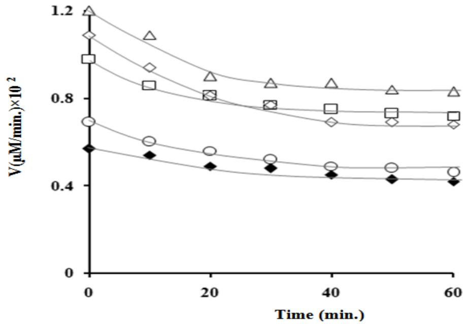
Figure 4. Stabilities of peroxidase at different pH when exposed for one hour at 10 minutes time intervals. (pH 4.0 (○), 5.0 (◇), 6.0 (△), 7.0 (□), 8.0 (◆))
