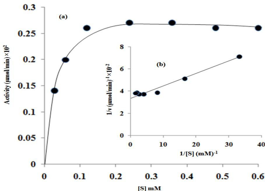
**Figure 2.** (a) Michaelis-Menten and (b) double-reciprocal plots for the peroxidase obtained from the juice of *B. vulgaris* (beet) using hydrogen peroxide as the variable substrate
