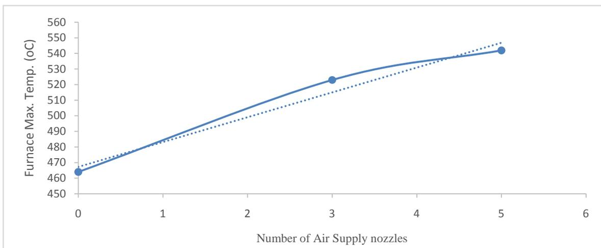
Figure 3. Variation of Air flow with maximum furnace temperature
