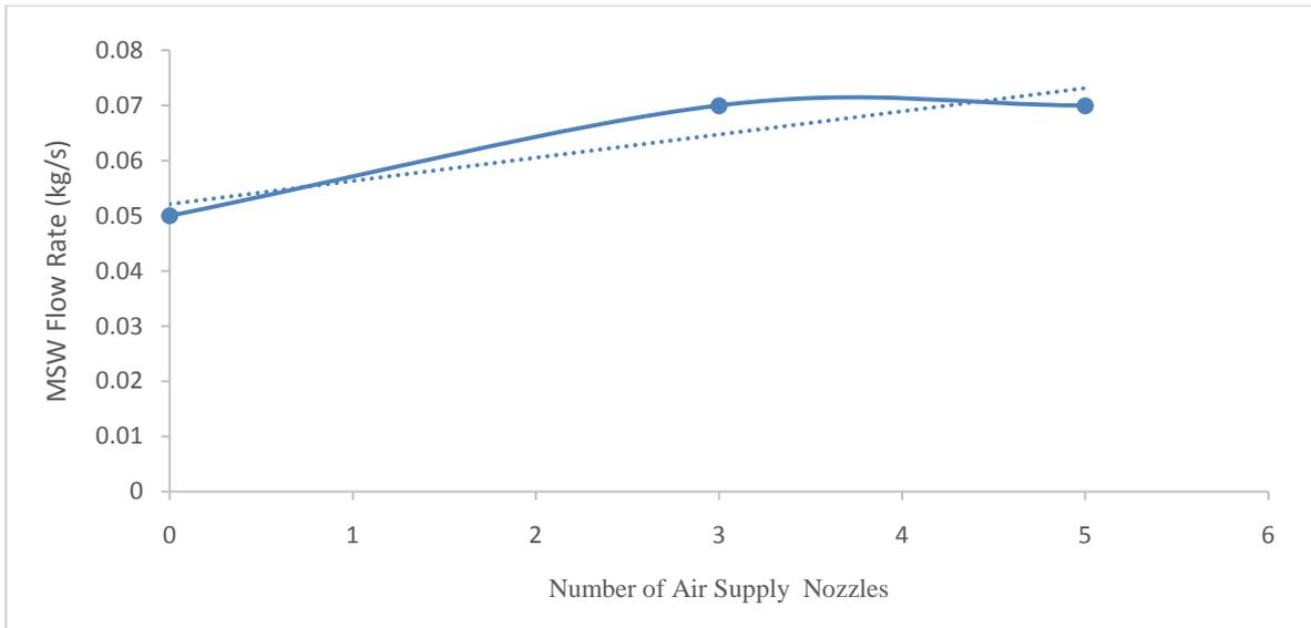
Figure 4. Variation of MSW Flow rate with respect to Air flow
