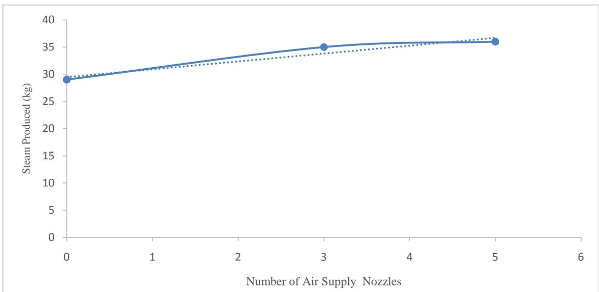
Figure 6. Variation of Air flow with steam produced
