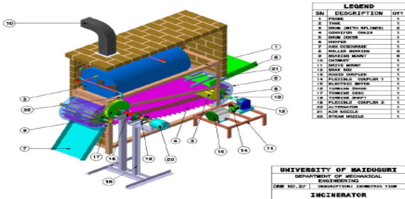
Figure 2. Schematic diagram of the Incinerator Set-up
