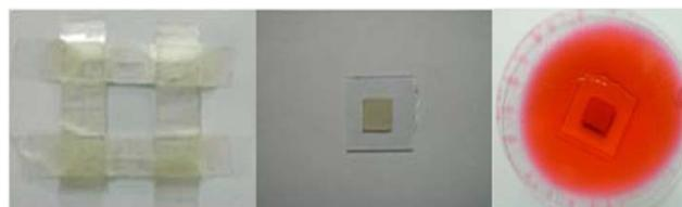
Figure 1. Shows the fabrication of dye sensitized sample by doctor-blade method
