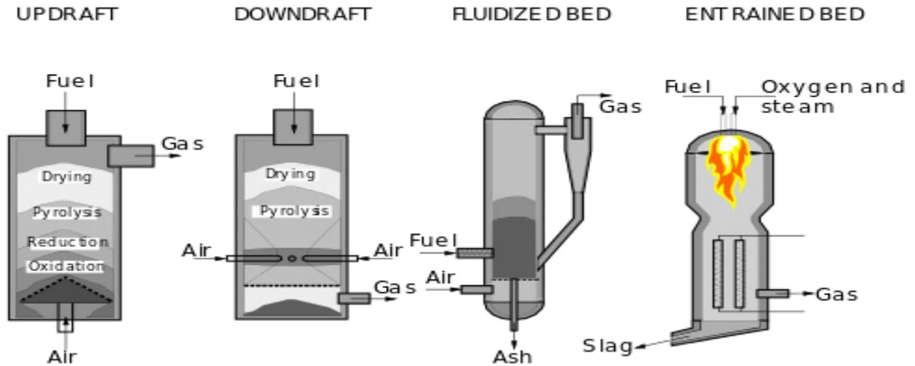
Figure 3. Main types of gasifier reactors [63]
