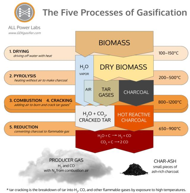
Figure 1. Reaction zones in a Downdraft Gasifier [54]
