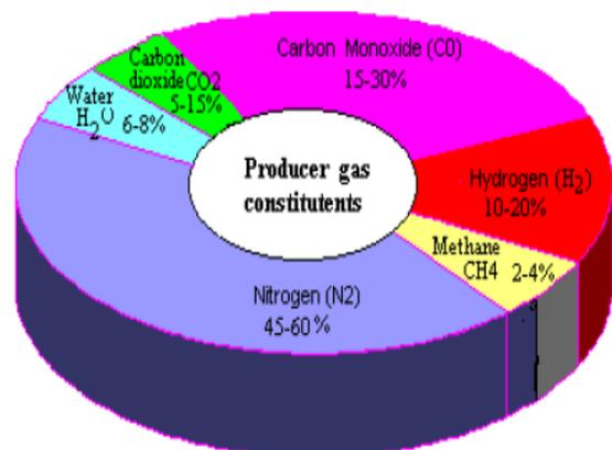
Figure 2. Syngas yields from gasification process [57]
