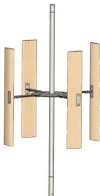
Figure 6. 3D geometric model of the H-Darrieus turbine
