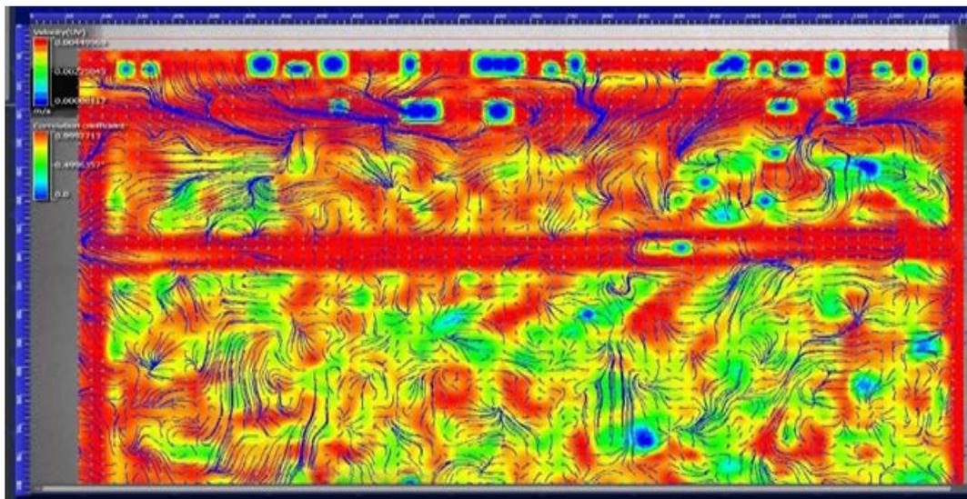
Figure 7. Correlation coefficient (region between the lower tray and upper tray)
