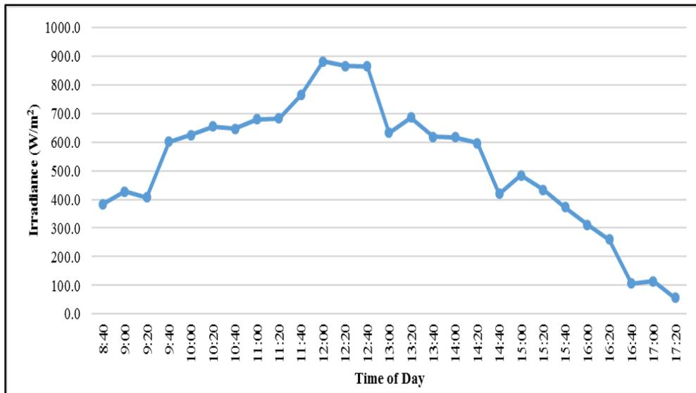
Figure 12. A graph of Irradiance (W/m<sup>2</sup>) against time of drying
