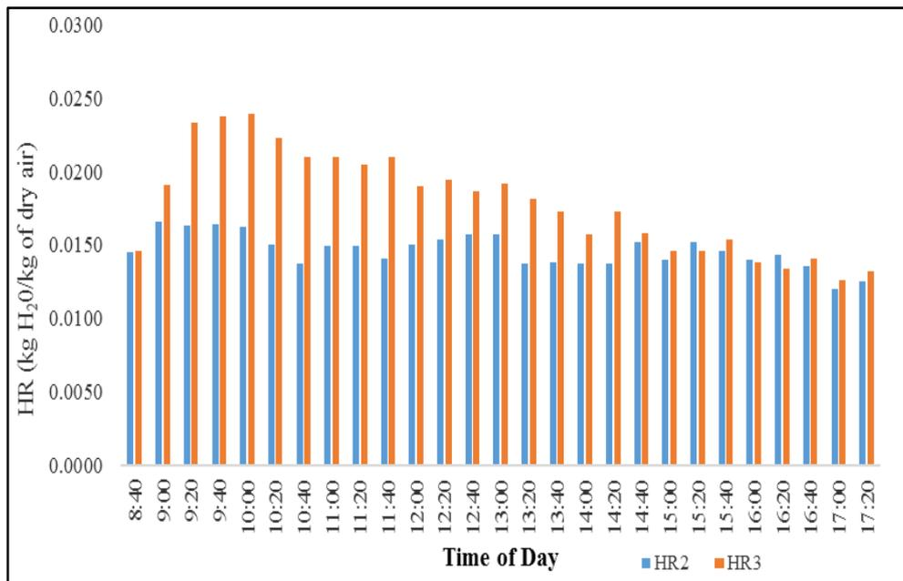
Figure 14. A graph of Humidity Ratio(HR) against time of drying
