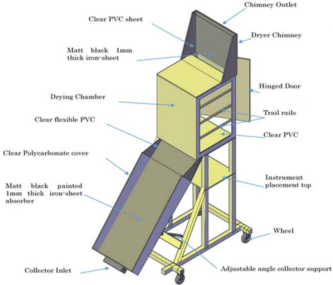
Figure 2. Modified Design solar dryer for PIV study
