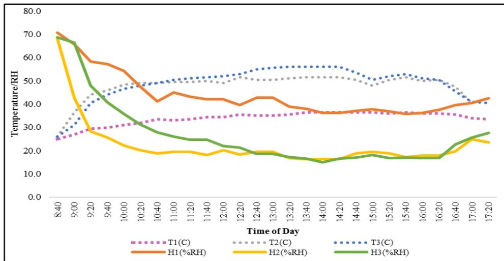
Figure 13. A graph of Temperature and Relative humidity against time of drying
