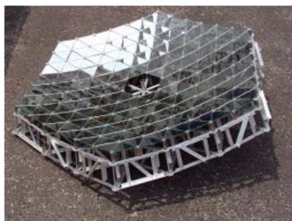
Figure 1. Solar concentrator prototype
