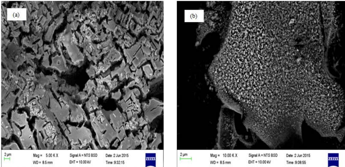
Figure 2. SEM micrograph of (a) dip coated  $\text{TiO}_2$ - bound,  $\text{CuFeMnO}_4$  paint on textured aluminum surface at X 5000 magnification (b) porous block of the  $\text{TiO}_2$ - bound,  $\text{CuFeMnO}_4$  paint coating formed on the textured aluminum surface taken at X 10 000 magnification
