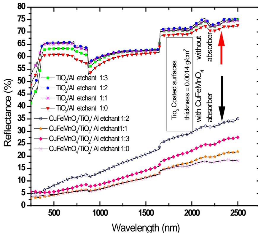
Figure 3. Reflectance spectra for; (i)  $\text{TiO}_2$ - coated textured aluminum surface (top), and (ii) dip coated  $\text{TiO}_2$ - bound,  $\text{CuFeMnO}_4$  paint on textured aluminum surface (bottom)
