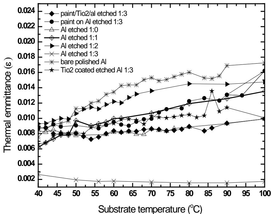
Figure 4. Thermal emittance of aluminum taken at  $24^\circ\text{C}$
