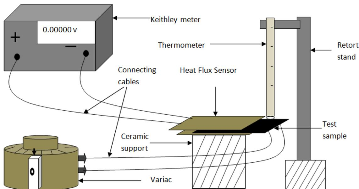
Figure 1. Set up for thermal emittance measurement
