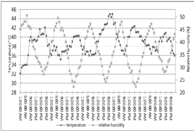
Diagram 3. the results of the environmental measurement of the air condition inside the summer place that is not connected to shevadun
