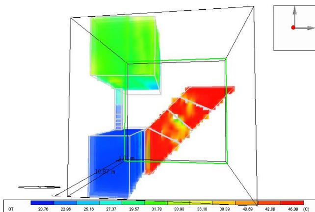
**Figure 12.** the distribution of the air temperature in the studied model at 3 P.M in August
