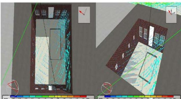
Figure 5. the distribution of the wind speed vectors at 3 A.M in August at the central yard
