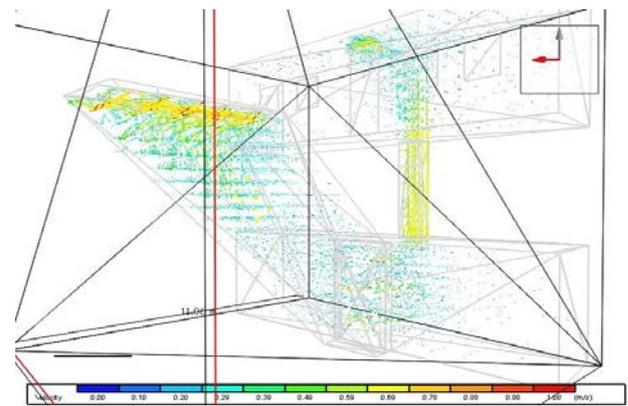
Figure 6. the distribution of the air flow velocity at 3 A.M in August in the studied model
