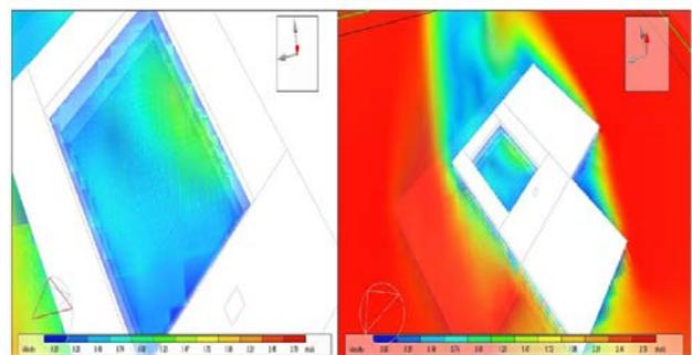
Figure 10. the distribution of the wind velocity at 3 P.M in August around the building and the central yard
