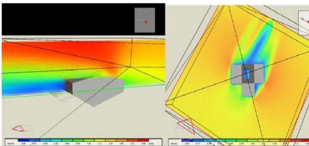
Figure 4. the distribution of the wind speed at 3 A.M in August around the building
