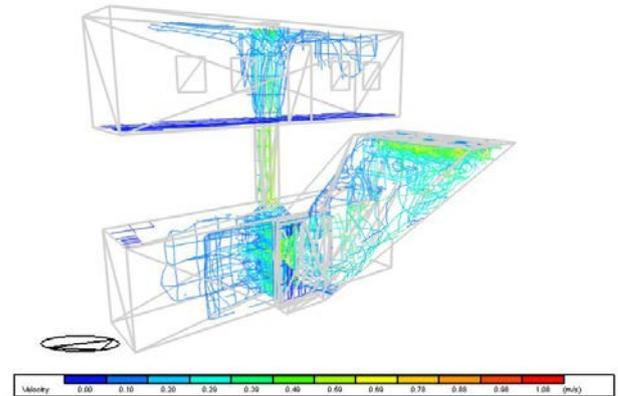
Figure 9. the is velocity and the direction of air flow in the studied model at 3 A.M in August
