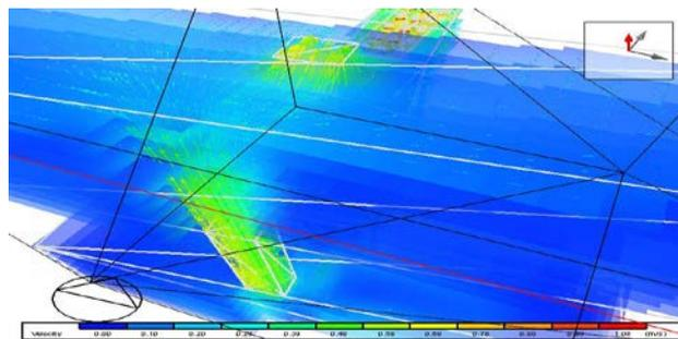
Figure 8. the distribution of velocity in the trapdoor on the roof at 3 A.M in August
