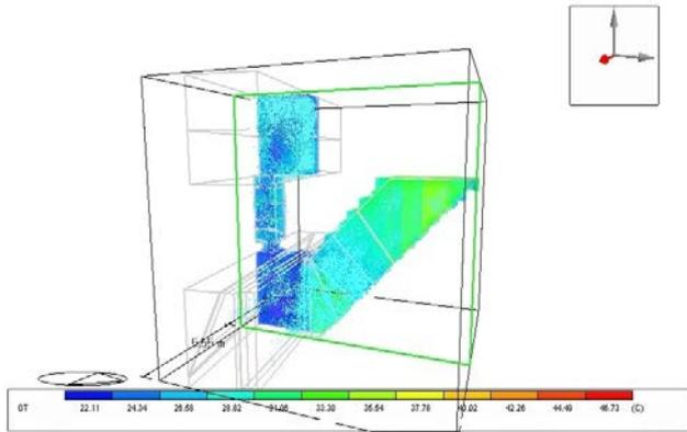
Figure 7. the distribution of the temperature in the studied model at 3 A.M in August
