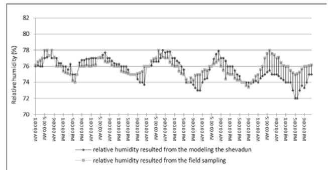
Diagram 7. the comparison of the relative humidity resulted from the modeling the shevadun
