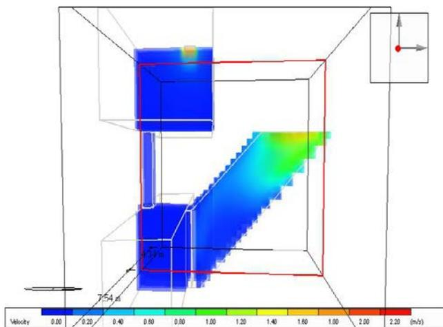
**Figure 11.** the airflow velocity distribution at 3 P.M in August in the studied model
