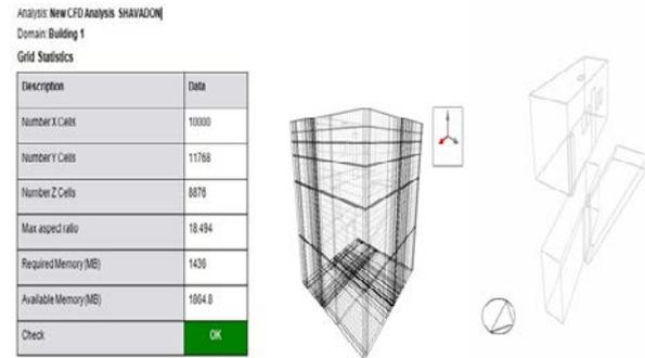
Figure 3. the characteristics of the built model in the Design builder software to perform the CFD calculations
