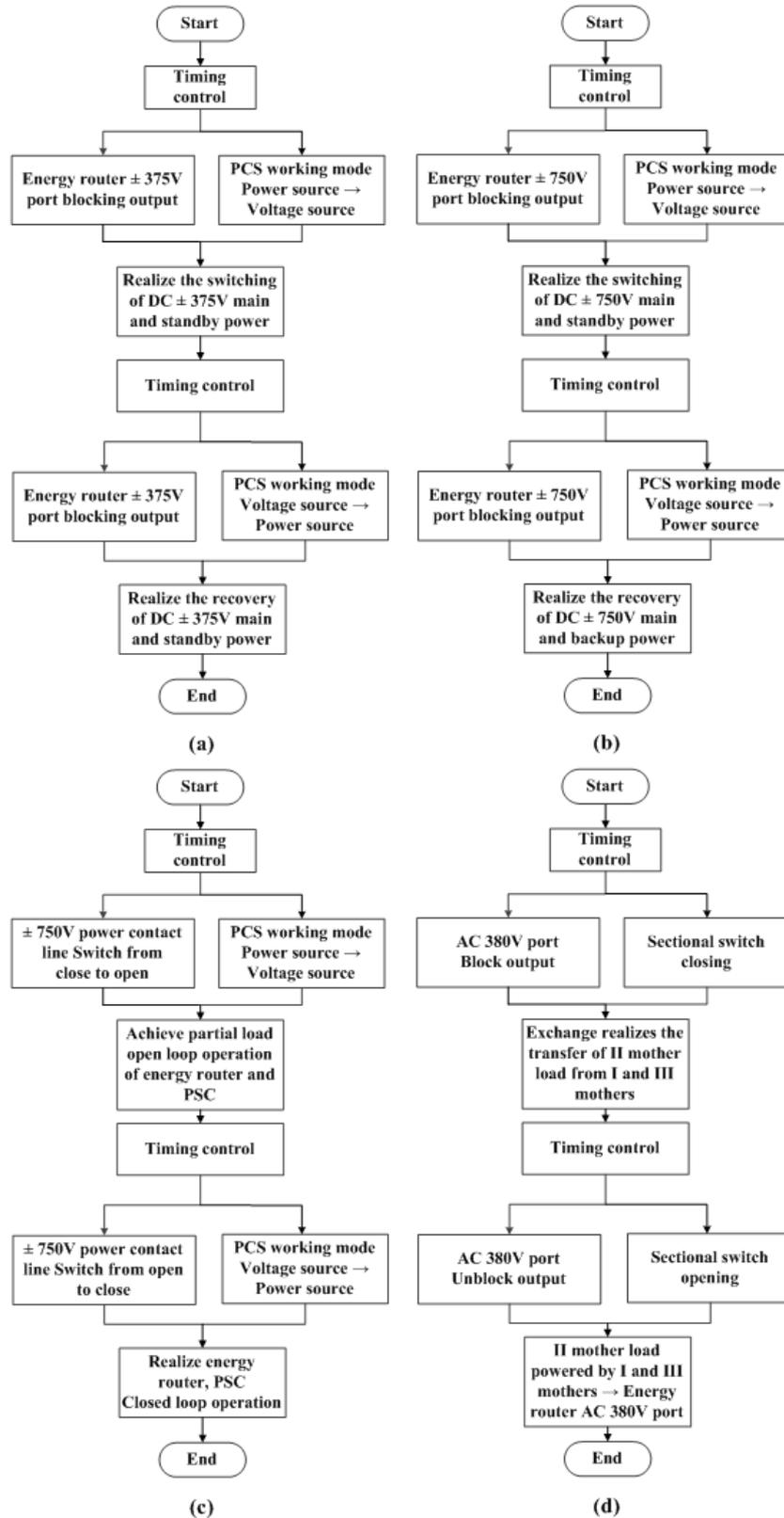
Figure 5. Flow chart of coordinated control method when operating mode is switched
