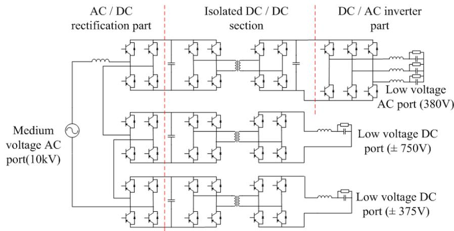
Figure 3. Topology of four-port energy router
