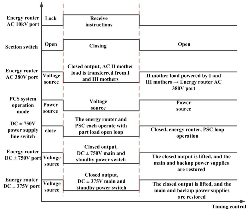
Figure 6. Time sequence diagram of coordinated control of AC/DC distribution network based on four-port router
