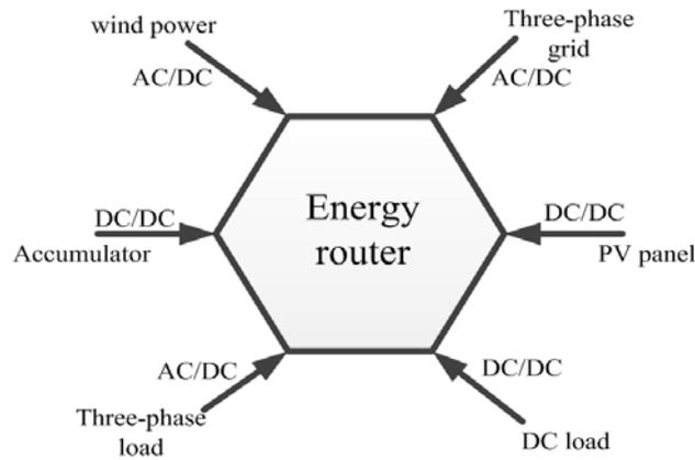
Figure 2. Conceptual graph of energy router
