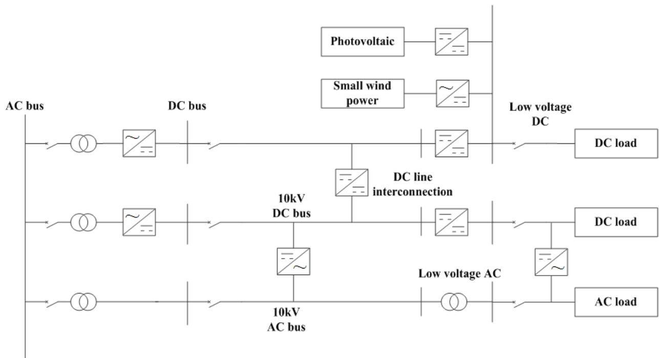
Figure 1. Typical Network Form of Medium Voltage AC/DC Distribution Network with DC Network
